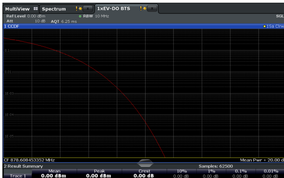
Figure 3-26: CCDF measurement results in the 1xEV-DO BTS application
